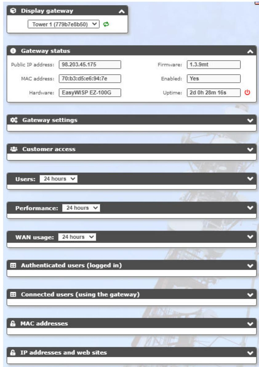
The easyWISP gateway configuration includes a list of parameters that can be configured via the Cloud for each easyWISP access controller. The parameters are listed below:
